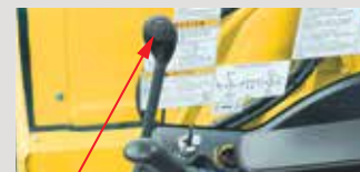
● Travel speed select switch The travel speed select switch is placed on the dozer lever and it allows selecting the travel speed.
