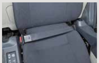
● Retractable seatbelt requires no manual adjustment
